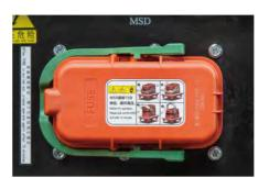
Both the battery and junction box have MSD(Manual Service Disconnect) maintenance switches to enable one-click power-down and safer maintenance.
